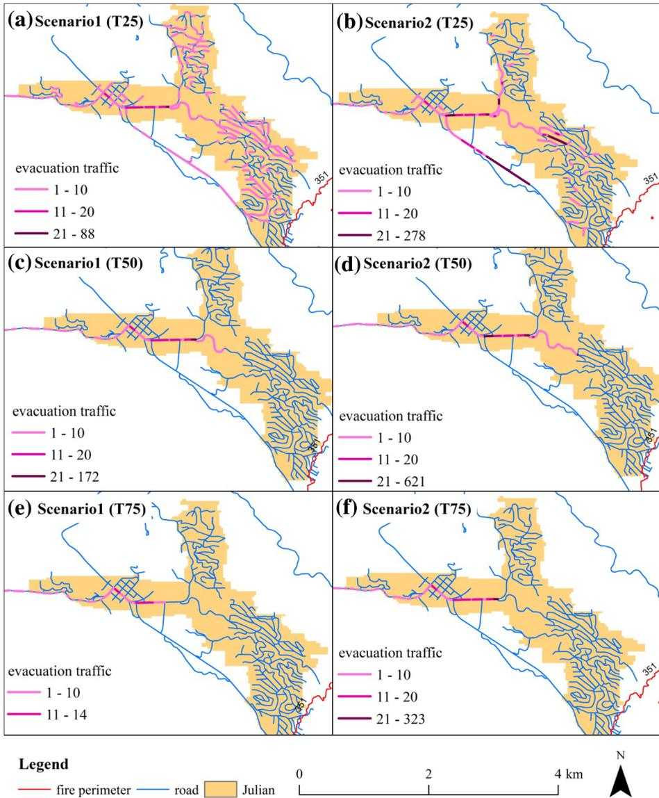
**Figure 12. The evacuation traffic for scenario 1 and 2. The evacuation traffic when the fire reaches the community was mapped out separately for each scenario and overlaid with the fire perimeters and road network data. More vehicles will be located closer to the fire front for a larger evacuation traffic demand. And a larger buffer can provide more time for evacuation but might cause early evacuation and disruptions.**
