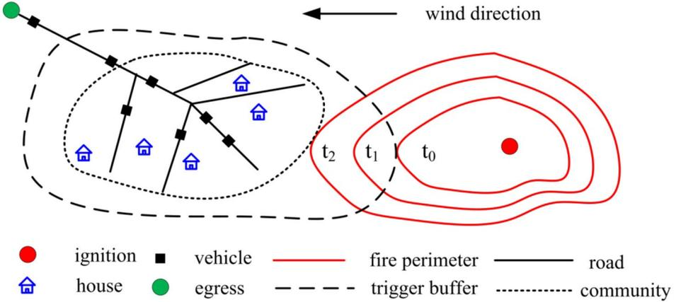
**Figure 7. The conceptual diagram of the evaluation procedure [51]. The fire starts at the ignition and spread towards the community. When the fire reaches the trigger buffer at  $t_0$ , the residents will be notified to evacuate. The evacuation traffic will be mapped out when the fire reaches the community at  $t_2$  to evaluate the effectiveness of the trigger buffer used during evacuation.**
