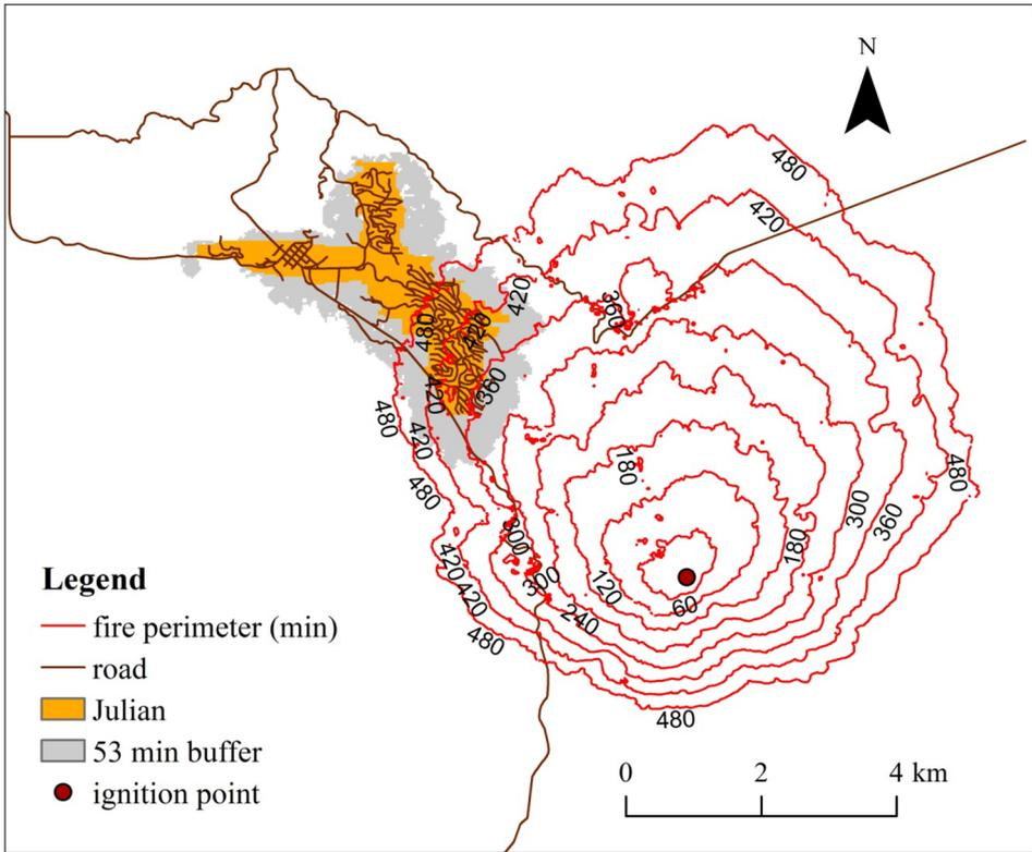
**Figure 11. Fire perimeters from wildfire simulation [51]. We derived fire perimeters from wildfire simulation and overlaid the perimeters with other datasets. Note that the perimeters are skewed along the wind direction while the trigger buffer is skewed against the wind direction.**
