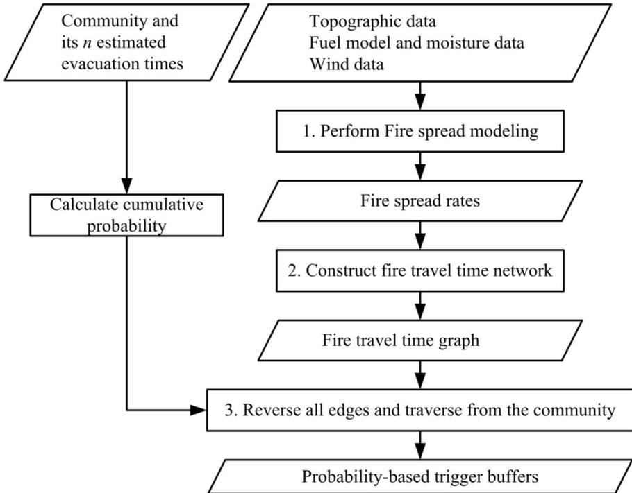
**Figure 6. The workflow of creating probability-based trigger buffers [51]. The ETEs derived from traffic simulations have their corresponding cumulative probability values and are used as the input time for trigger modeling. A trigger buffer based on fire spread rates is generated for each input ETE, and thus each trigger buffer is also associated with a probability value.**
