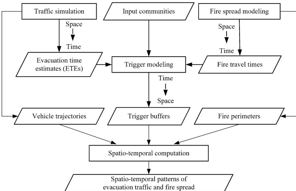
**Figure 2. A spatiotemporal GIS framework for model coupling [51]. Traffic simulation is used to derive ETEs, which can be used as the input for trigger modeling. Fire spread rates and travel times can be calculated using fire spread modeling. Finally, we couple fire spread and traffic simulation models to examine the spatio-temporal patterns of fire spread and evacuation traffic.**
