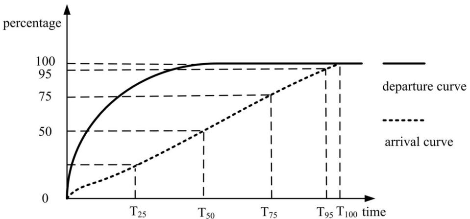
**Figure 4. An illustration of the derived four ETEs [51]. Specifically, we calculate the time taken when 25, 50, 75, and 95% of the evacuees have arrived at the safe places during the evacuation for each run of traffic simulation. If we perform traffic simulation  $n$  times, we can derive  $n$  sets of these four ETEs.**
