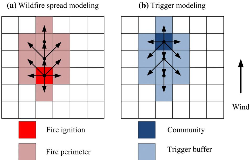
**Figure 1. Illustration of wildfire spread and trigger modeling: (a) A demonstration of wildfire spread modeling; (b) A demonstration of trigger modeling [51]. Wildfire spread modeling uses the shortest path algorithm and the fire spread rates in eight different directions in one cell to derive fire travel times for each raster cell. Trigger modeling reverses edges in opposite directions and also employs the shortest path algorithm to create a raster buffer for a threatened community.**
