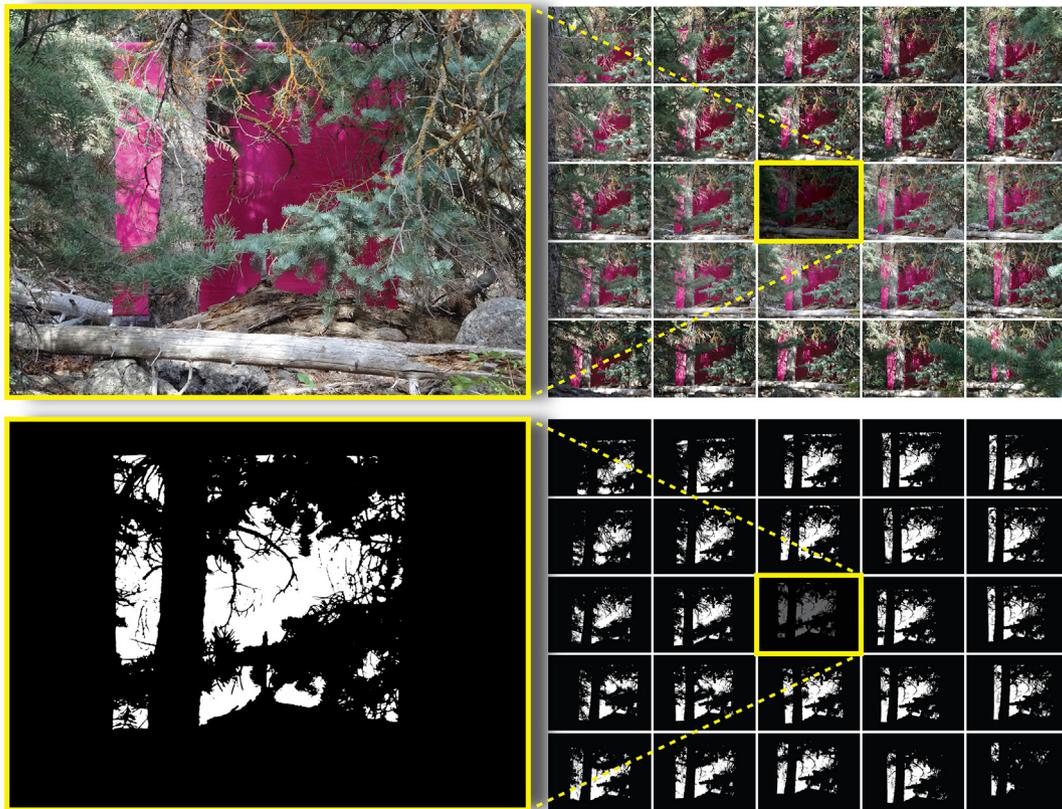
Fig. 6. Cover board photo classification example results. In the lower two panels, white indicates pixels classified as “board” and black indicates pixels classified as “non-board”.
