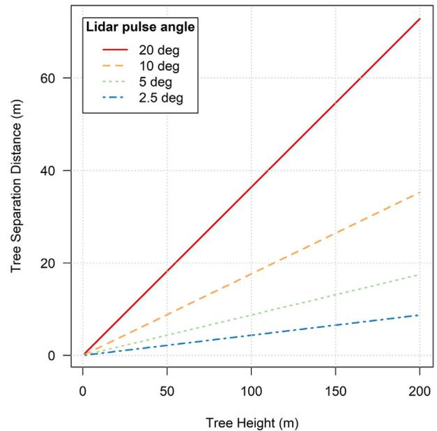
Fig. 2. The relationship between tree height and theoretical tree separation distance under which individual lidar pulses could interact with multiple trees at various scan angles.
