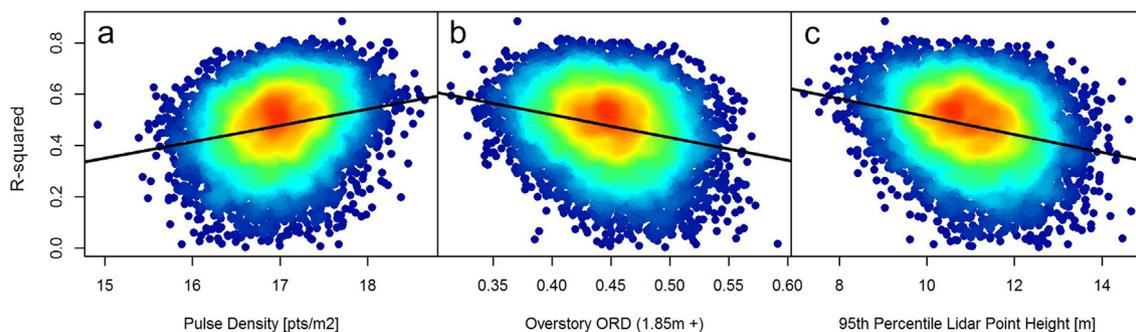
Fig. 8. The bootstrapped effect of lidar pulse density (a), overstory canopy density (as approximated by lidar overall relative point density of all points higher than 1.85 m) (b), and canopy height (as approximated by 95th percentile of lidar point return height) (c) on the ability of lidar to model understory cover (as approximated by the amount of variance in cover board cover explained by lidar understory normalized relative point density).
