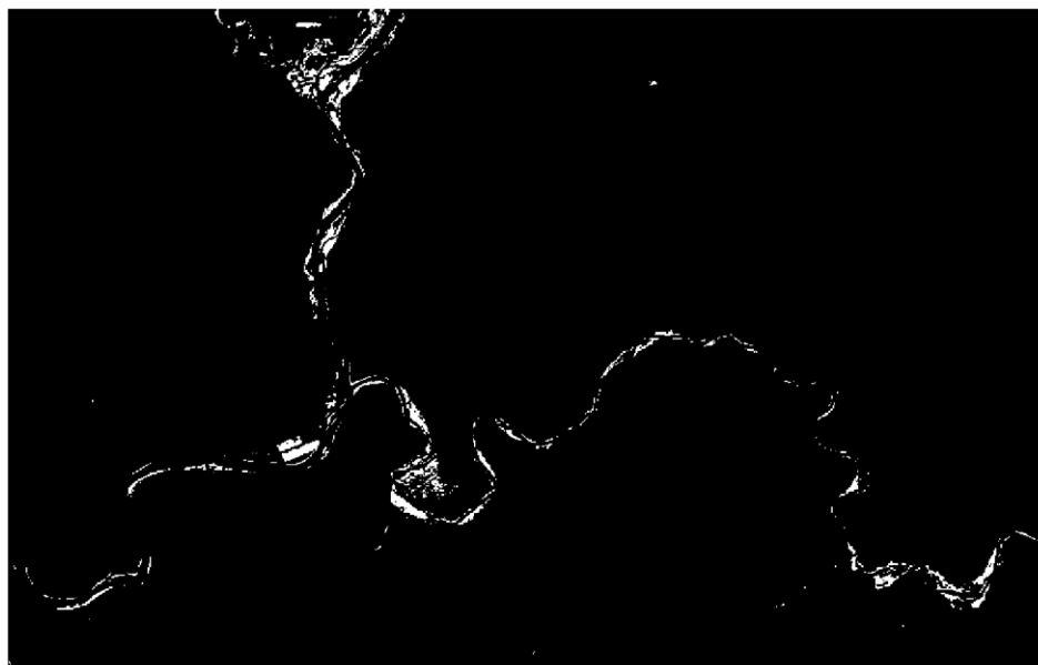
Fig. 5. Defoliated areas in the 2007 ASTER image (white) were calculated as pixels with a 0.1 or greater decrease in NDVI and a 2006 NDVI of at least 0.3. The area shown corresponds to the same area in Fig. 3.
